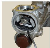
The GSS-2 module fits in the Type 9 gearbox extension housing and is wired to the car's ECU via a waterproof connector. A minor modification is required to the gear lever/selector rod coupling and the ECU or digital display gear selector voltage settings may need to be adjusted in order to read and display the selected gear correctly .
